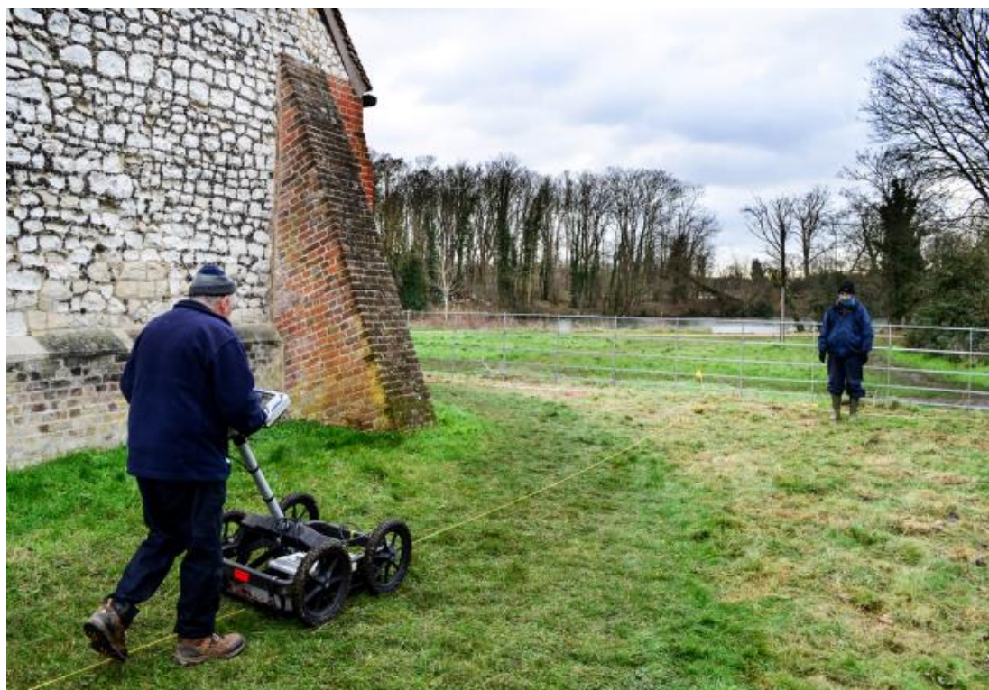
Figure 2: the GPR in action at Boveney. Photo: © Mike Smith.
